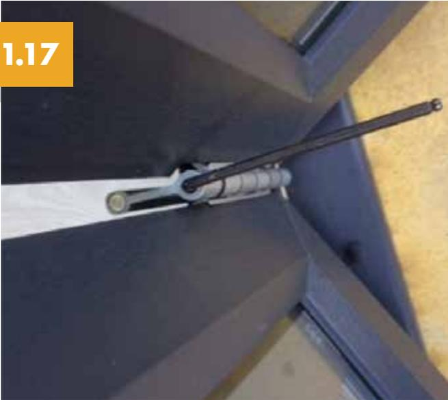
Roller adjustment is achieved by loosening the grub screw, then using a 5mm Allen key. Make the required adjustment and then retighten the grub screw. (8mm of adjustment is available).
