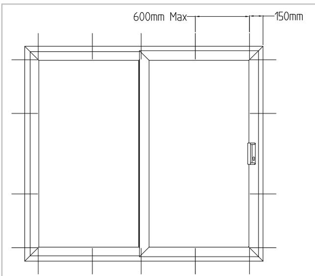
If fixing cleats is the chosen method of installation they should be attached to the outer frame starting at 150mm from the corner and thereafter at a maximum of 600mm centres. The cleats should be screwed into the mainframe in the central reinforcing chamber. Direct fixings should be in the same centres as above.
