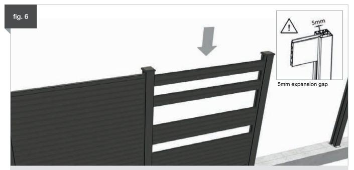
Fence sections are assembled, post skirt (if required) bottom rail, required number of panels, then insert top rail. Secure with L shaped block, if required. Add infills to unused post slots and then apply caps to posts. Caps can be secured by screws in the side if needed. **NOTE:** A 5mm expansion gap is important between the board and the post.
