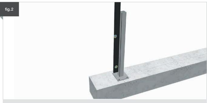
Ensure the insert is plumb and secure. Use steel shims / packers if required.
