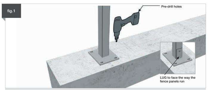
Before starting - ensure the wall or footing is in adequate condition. Pay particular attention to where you place the LUG this is where you will need to secure the post to the post mount.
