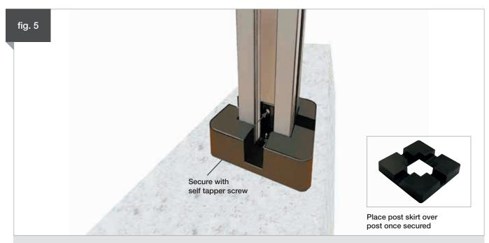
To secure the fence post to the fence base plate, drill through the inside of the post and insert a self tapper. Make sure the LUG is facing the correct way when placing the post - this will face the way the fence panel runs.
