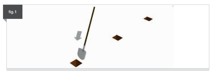
Dig a hole using a narrow shovel or Fencers graft to a depth of 600-850mm depending on the softness of the ground. Ensure the base of the pit is level.
