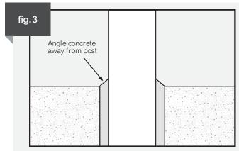
When finishing the concrete around the base of the post, angle the concrete away from the post to allow rainwater to drain away easily.
