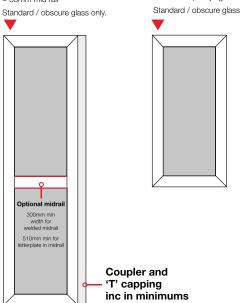
220mm no mid Min 250mm mech mid Min 300mm welded mid Midrail = 70mm as standard 115mm optional and required for letterplate
