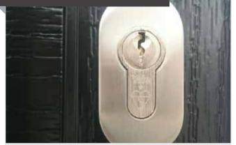
These should be fitted using the screws provided and pilot drilled using a 2mm drill bit. Never drill more than 10mm into the door leaf as damage to the lock can occur if you drill deeper.
