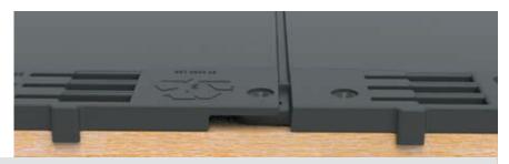
Each tile has two detachable nibs (F) at the top. These are used to hook the tile over the batten. When a batten has been fitted out of alignment or there has been some movement after fitting, the installer can break the nibs off as required if they find that the nibs no longer hook over the batten.
