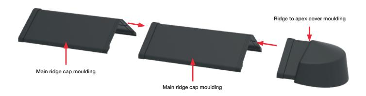
Starting at the right hand side loose fit the ridge to apex cover moulding over the hip to ridge apex. Then loose fit the ridge cap moulding over the ventilated ridge roll and then interlock with the next ridge cap.
