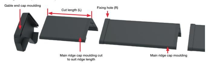
Lay out and interlock the main ridge sections together loosely along the full width of the roof. When correctly aligned permanently fix into place using the bedded batten as a fixture point for the 90mm x 6.3mm Stainless Steel Pozi Pan Self Tapping (ENVSCREW90) required to permanently fix two ridge sections together. Start the mechanical screw fixing procedure from the right hand gable end, using the fixing hole (R) on the apex at each end.
