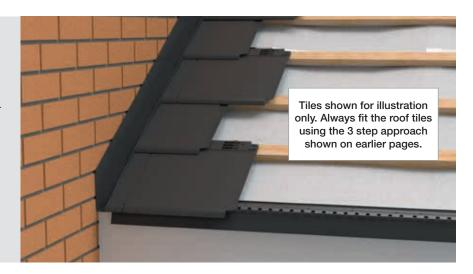
Leave a gap of 38mm between the abutment wall edge and end of roof tiles.
