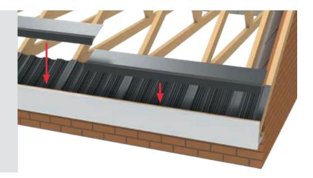
Note: At ends overlap each universal felt support tray by a minimum of 100mm to ensure water tightness is maintained.
