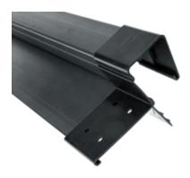
To finish gable ends it is recommended that the continuous dry fix verge (ENV3MDV) is used. This is fitted over the top of the battens and runs along the top edge of the end rafters at gable ends. Use dry verge brackets (ENVDVB) to join lengths of dry verge if required.
