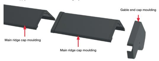
Starting at the right hand side of the roof, align and loosely fit the ridge cap mouldings over the ventilated ridge roll by interlocking the ridge sections together. At the gable the end cap envelopes the mitred dry verge before interlocking with the end ridge section (see illustration).
