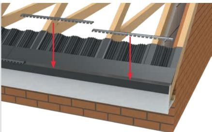
Starting at the right hand gable end verge, run through the full roof width with eaves bar/starter rails ENVEB then mechanically fix with stainless steel screws.
