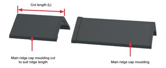
If the cut length (L) is less than half the length of the ridge cap moulding it is recommended that you cut two ridge cap mouldings and space accordingly.
