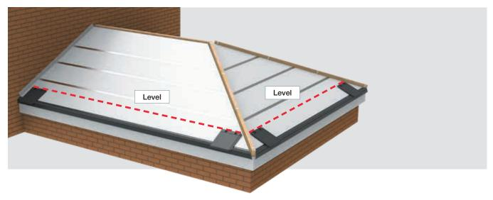
In a warm roof construction the Envirotiles are fixed directly onto the plywood roof face panels. There are no battens so it is very important that the installer checks that the first course line is level. The easiest way to do this is to clip a single tile into the starter rail at each end of each roof face and run a line as shown. Adjust the line so it is level - the starter rail allows for some tile adjustment.
