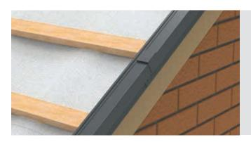
Fix a bracket clip, if required, with screw fixings ENVDVB, to join lengths of continuous dry fix verge when rafters are longer than 3m in length.
