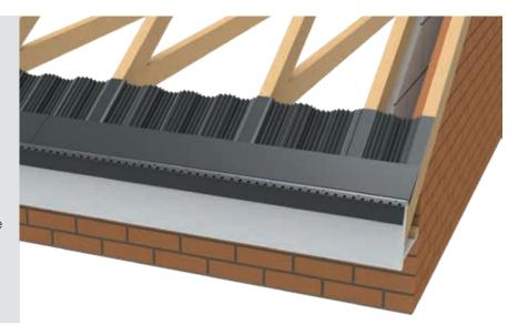
For abutment wall roofs ensure that the final Starter Rail located next to the wall provides a gap of 40mm away from the wall edge.
