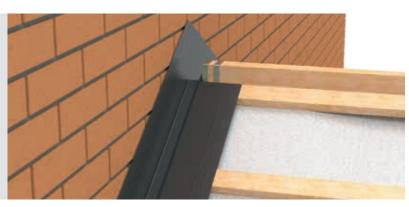
After fixing the abutment soaker correctly overlap/install the wall flashing to make watertight, as illustrated.
