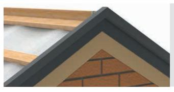
At the apex centre mitre cut and abut to the continuous dry verge unit to the correct pitch angle in readiness for the gable end cap to be fixed.
