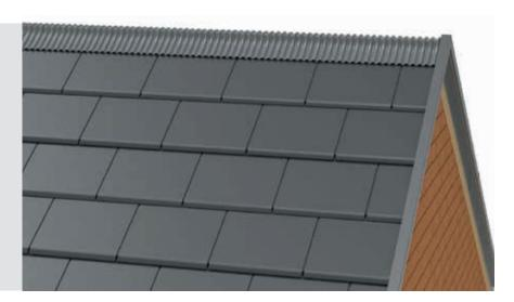
Run the ridge roll so that it buts up flush with the abutment wall ensuring an overlap at the top edge of the soaker channel.
