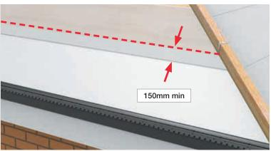
Use Duo Plus Tape (ENVTAPE) to seal the overlap layers.
