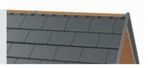
Place the ridge roll over the centre of the bedded batten and lay over the ridge apex ensuring the roof tiles are used as a substrate and overlapped by a minimum distance of 100mm either side of the apex.
