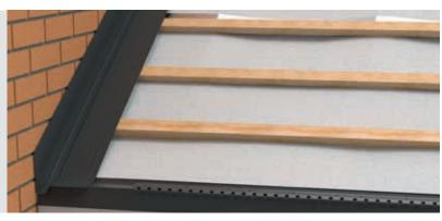
When the abutment soaker is secured, fit the final starter rail as shown, screwing through the abutment soaker.
