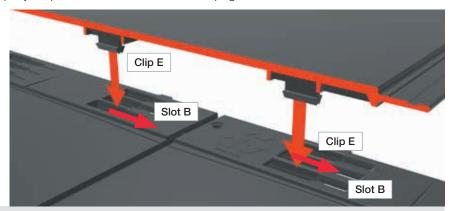
Envirotiles are clipped together using the two clips on the underside at the bottom of the tile (E) clipping into the slots at the top of the tile on the course below (B). Note that the tile must be aligned, then pushed down, then the tile is slid to the right to lock into the clip. The sliding action also locks the connecting strip into the adjacent tile slot.
