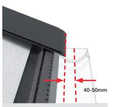
Note that the distance between the leading edge of the tile should be located approximately centre of the fixed gutter by a distance of 40-50mm.
