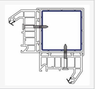
To do this you remove the beads using the pull straps (sides first then top and bottom) and make a note of where they go and which window they are from (as they are all cut bespoke).
