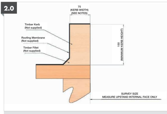
Prepare a 75mm width timber kerb for the rooflight (not supplied with rooflight).
