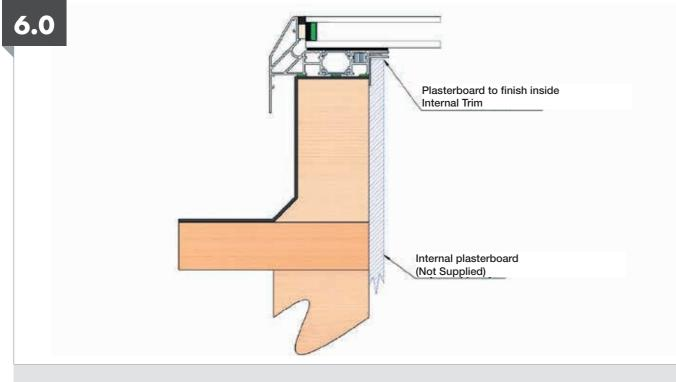
After securing the rooflight in position, proceed to install and fix all internal plasterboards ensuring plasterboards finish inside ET12564-Internal Trim.
