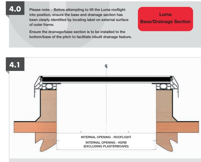
Observing necessary risk assessments, method statements, Health & Safety requirements and safely utilising all appropriate lifting equipment and PPE, carefully bring the rooflight into position aligning the rooflight centrally over the kerb internal opening.
