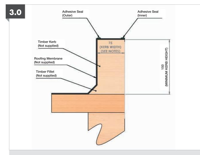
Before lifting the rooflight into position apply adhesive seals to the kerb. Apply two (2) generous beads of adhesive seal around and to the top surface of the kerb. Apply one bead to the internal and external perimeters of the kerb.
