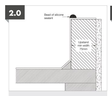
Ensure the kerb is clean and free from debris, then run a silicone bead around the external edge as shown above.
