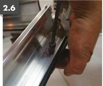
Using 2 x CRS8624S single studs, secure each hip to the spider casting. The body of the stud should locate between the retaining ribs on the lower casting face to stop the stud from spinning.
