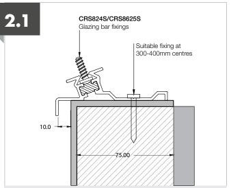
Ensure correct amount of glazing bar fixing studs are slid into the ring beam before any fixing commences. Position the ring beam so an equal overhang is achieved around perimeter and fix using suitable 5-6mm fixings at 300-400mm centres (starting and ending 100mm away from internal corner of the ring beam).
