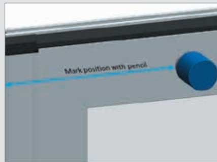
C. Mark position on swing door
