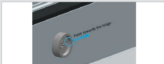
E. Position anti-rotation point
