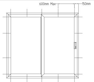
If fixing cleats is the chosen method of installation they should be attached to the outer frame starting at 150mm from the corner and thereafter at a maximum of 600mm centres. The cleats should be screwed into the mainframe in the central reinforcing chamber. Direct fixings should in the same centres as above.
